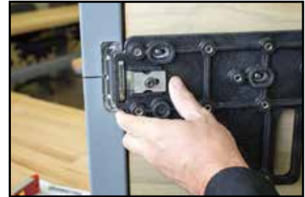
Step 8 - Test the position of the bolt and strike by moving the simulated bolt in and out of the strike.
